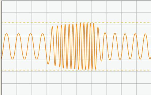
Current waveform in sudden acceleration/deceleration at 0.5Hz
