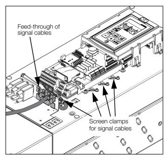
Fig. 64 Connecting the control signals, VFX model 48-142 to 48-365 frame size E2, F2 and FA2 (principle drawing)
