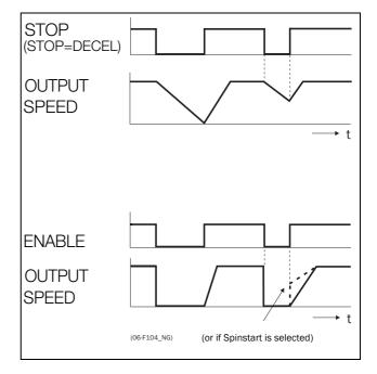
Fig. 71 Functionality of the Stop and Enable input
