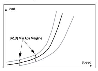
Fig. 123 Load Curve R with Min ABS margin.
