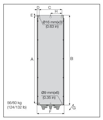
Fig. 18 Emotron VFX Model 48-090 to 175 (Frame size E).
