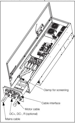
Fig. 45 Connection of lower mains and motor cables.
