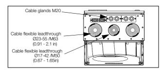
Fig. 21 Cable interface for mains, motor, DC+/DC-, brake resistor and communication, Emotron VFX Model 48-210 to 295 (Frame size F), Emotron VFX Model 69-082 to 200 (Frame size F69).
