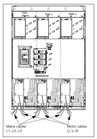
Fig. 52 IP20 module sizes I/I69 with qty 3 x 3 Mains cables and qty 3 x 3 motor cables.
