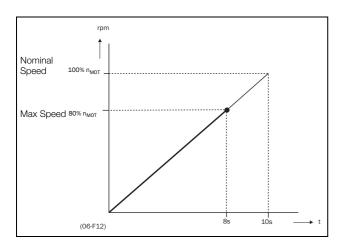
Fig. 98 Acceleration time and maximum speed
