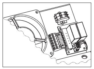
Fig. 160 Connection of safe stop option in size E and up.
