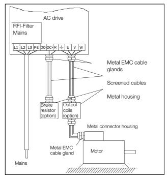
Fig. 66 Connection of mains and motor cables.
