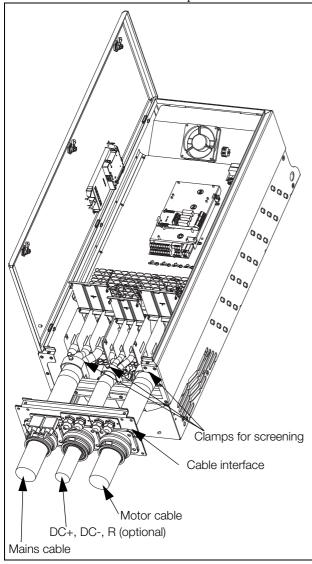
Fig. 44 Connecting motor and mains cables.
