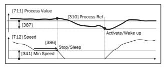
Fig. 112 PID Stop/sleep with normal PID
