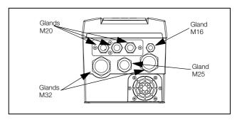
Fig. 6 Cable interface for mains, motor and communication, Emotron VFX Model 48/52-003 to 018 (Frame size B).
