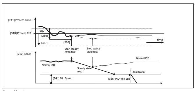
Fig. 114 Steady state test
