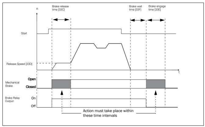
Fig. 103 Brake Output functions
