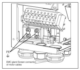
Fig. 32 Mains and motor connections, model 026-046, frame
