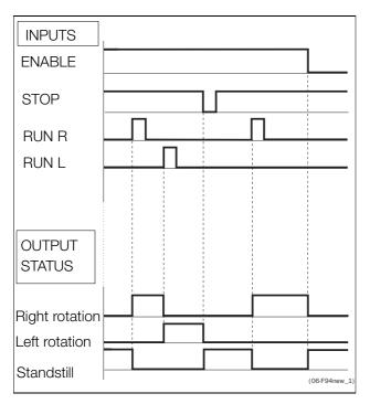
Fig. 74 Input and output status for edge-control
