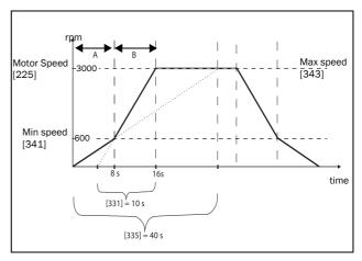
Fig. 100 Calculation example of accelerating times (graphics not proportional).
