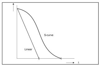
Fig. 102 Shape of deceleration ramp
