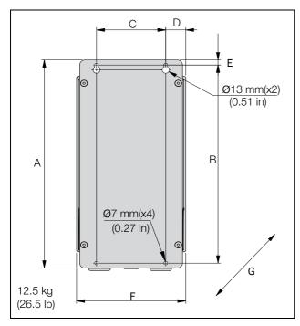
Fig. 5 Emotron VFX Model 48/52-003 to 018 (Frame size B).
