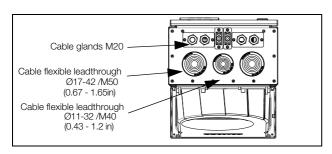
Fig. 19 Cable interface for mains, motor, DC+/DC-, brake resistor and communication, Emotron VFX Model 48-090 to 175 (Frame size E).
