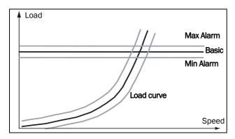
Fig. 122 Basic load type and Load curve
