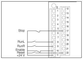
Fig. 72 Example of wiring for Run/Stop/Enable/Reset inputs
