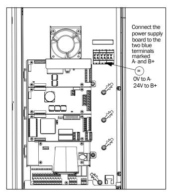
Fig. 158 Connection of standby supply option on frame sizes D, D2, FA, FA2, C69, D69, C2(69) and D2(69).
