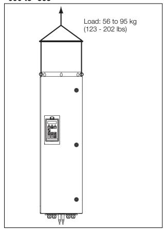
Fig. 2 Lifting AC drive model -090 to -365.
