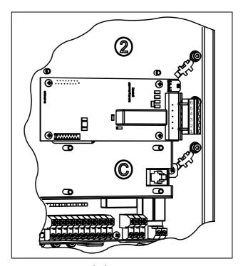
Fig. 159 Connection of safe stop option in size B - D.
