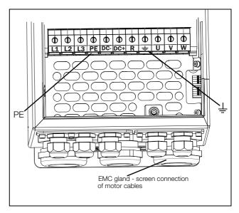
Fig. 35 Mains and motor connection, model 061 - 074, frame size D and model 69-033 to 69-058 frame size D69.
