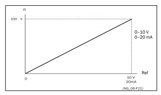
Fig. 127 Normal full-scale configuration
