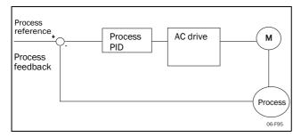
Fig. 111 Closed loop PID control
