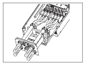
Fig. 48 All cables and cable clamps connected.
