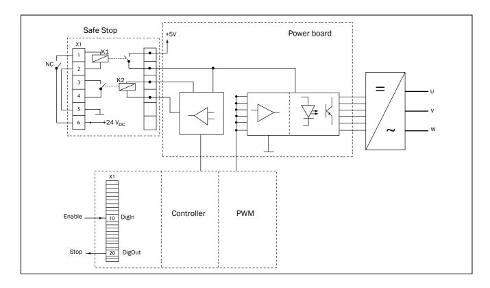
Fig. 161 Safe Stop connection
