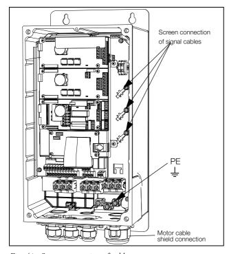
Fig. 41 Screen connection of cables.
