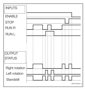
Fig. 73 Input and output status for level-control
