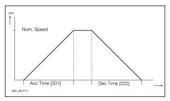
Fig. 99 Acceleration and deceleration times
