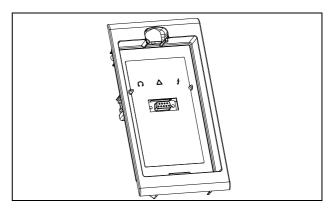
Fig. 77 RS232 connector behind the control panel
