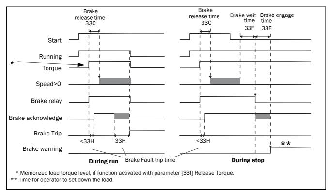
Fig. 104 Principle of Brake operation for fault during run and during stop
