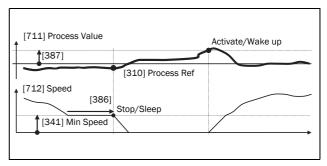
Fig. 113 PID Stop/sleep with inverted PID
