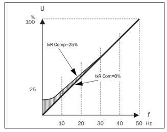
Fig. 108 IxR Comp at Linear V/Hz curve
