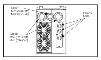
Fig. 9 Cable interface for mains, motor and communication, Emotron VFX Model 48/52-026 to 046 (Frame size C).
