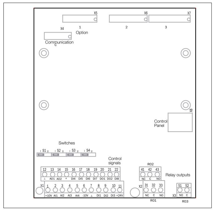
Fig. 56 Control board layout
