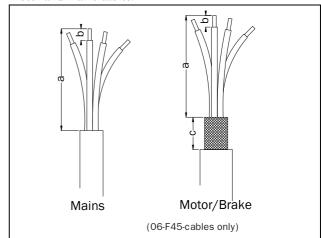
Fig. 53 Stripping lengths for cables
