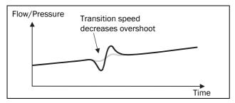
Fig. 120 Effect of transition speed
