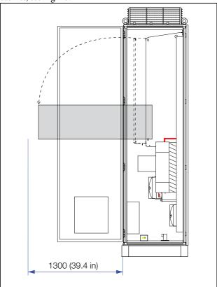
Fig. 28 Recommended free space in front of the cabinet mounted AC drive.
