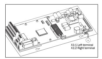
Fig. 157 Connection of standby supply optionon frame sizes B, C, C2, E, E2, F and F2.
