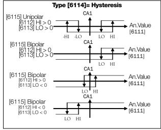
Fig. 136 Principle functionality of comparator features for "Type [6114] = Hysteresis" and "Polar [6115]".
