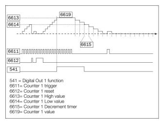
Fig. 141 Counters, operating principle.
