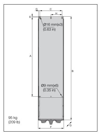
Fig. 25 Emotron VFX Model 48-365-54 (Frame size FA).
