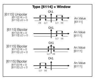
Fig. 137 Principle functionality of comparator features for "Type [6114] = Window" and "Polar [6115]".
