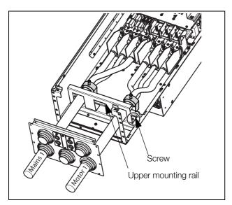
Fig. 47 Upper mounting rail mounted over the lower cables.
