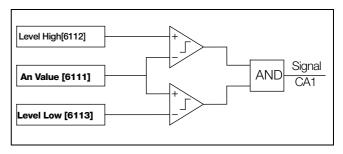
Fig. 133 Analogue comparator type "Window"
