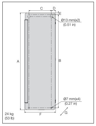
Fig. 8 Emotron VFX Model 48/52-026 to 046 (Frame size C).
