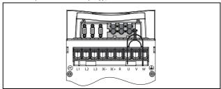
Fig. 17 Bottom view Emotron VFX Model 48-060 to 48-105 (Size D2), Model 69-033 to 69-058 (Frame size D2(69)), with cable interface for mains, motor, DC+/DC-, brake resistor and control.
