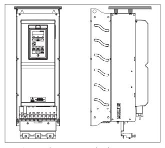
Fig. 162 Optional top cover mounted on frame size D2
