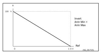
Fig. 129 Inverted reference
